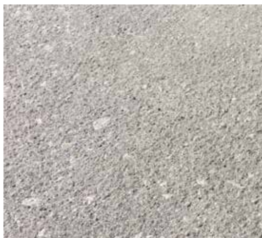
Profile of concrete after one pass with the HTC Ravager™
