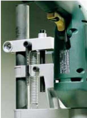
depth of cut set by depth stop
