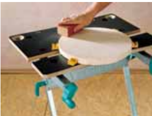
plastic jaws for securing the workpiece horizontally
