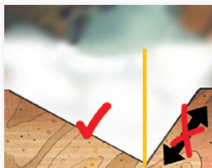
Unsurpassed precision – approved right-angled height adjustment. Distance of noches always constant irrespective of wood tolerances.
