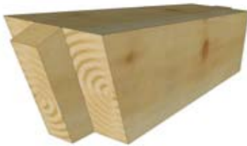
Tenon (with mitered shoulders)
