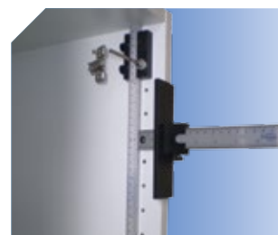
Drilling for placing invisible hinges.
