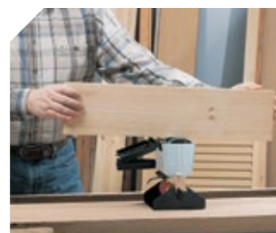
Gluing with the upper roller.
