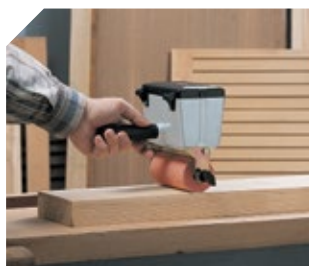
Gluing with vinyl (white) glues
