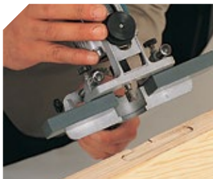
Placing hinges with the ZB93 head.
