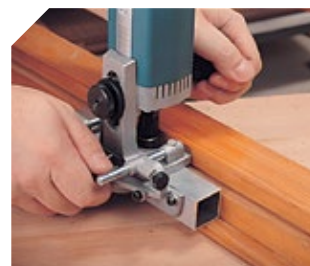
Slotting a window, lock side.
