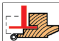
Slotting a window, hinges side.
