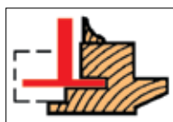
Slotting a window, flashing side.
