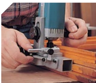
Slotting a window, flashing side.
