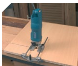
Trimming parallel slots.
