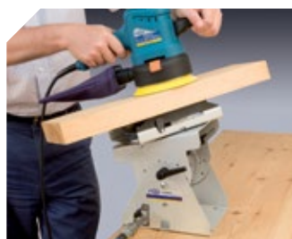
Folding and rotary adjustable support.
