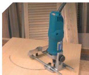
Trimming circular slots.
