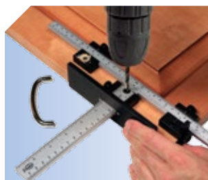
Drilling for door handles.
