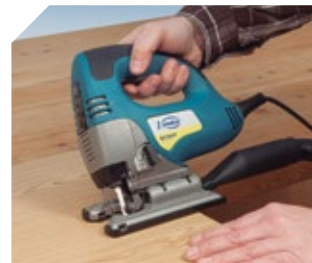
Base can be tilted from 0° to 45°.
