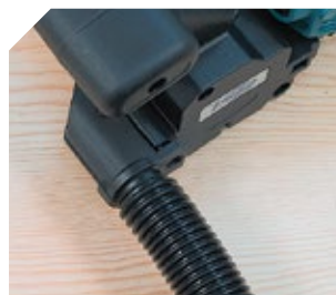
Dust collector connection.
