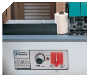
Electronic temperature regulation.
