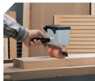
Gluing with vinyl (white) glues
