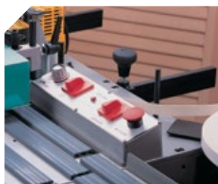
Safety control (STOP). Electronic temperature control.
