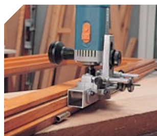
Slotting a window, hinges side.
