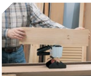
Gluing with the upper roller.
