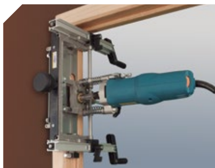
Making the upper recess on the frame.
