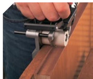
Banding the upper side of the lap.
