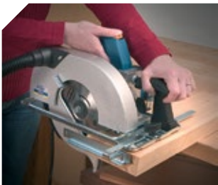
Performs cuts of up to 70 mm.
