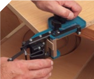
Cutting on both sides on straight panels.
