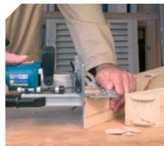
Stronger joints with No. 6 splines.
