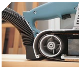
External dust collector connection on model LB31E.
