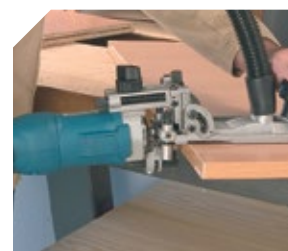
Trimming the edge with the straight bit.
