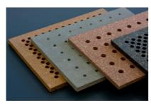
Demand for panels with superior visual appeal for interior and trade show construction has increased steadily in recent years. For these applications, we provide a factory perforated panel in four different standard versions. Products can be selected from 32 x 32 mm patterns with 8 or 10 mm holes and 16 x 16 mm patterns with 6 or 8 mm holes. The product can be shipped in grey simulated concrete
