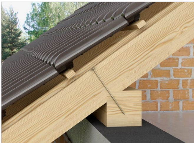
Joint between rafter and wall plate
