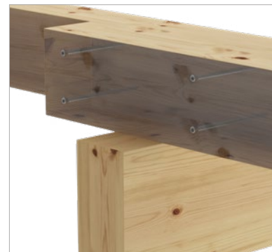
Joint between two passing-by beams
