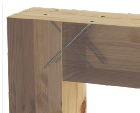
Joint between two girders
