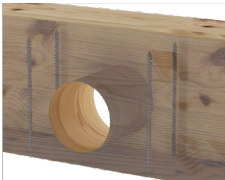
Reinforcement of beam in the point weakened by drill hole
