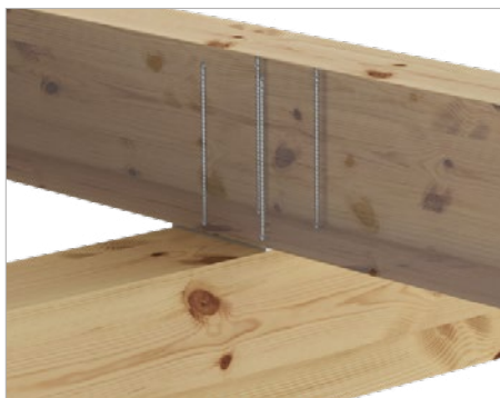
Reinforcement in the point of support
