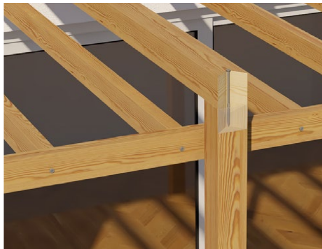
Joint between beams in pergola construction
