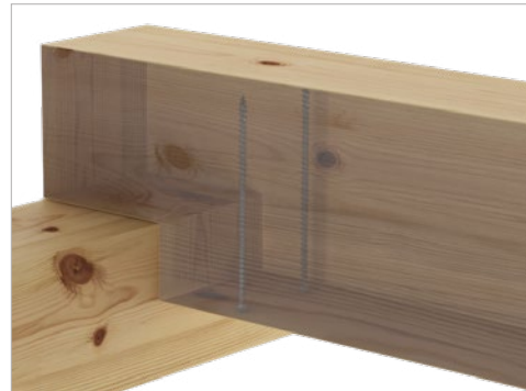
Protection against failure of notched beam
