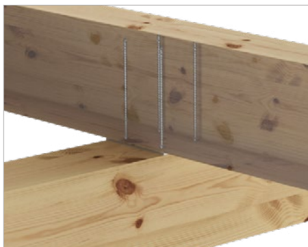
Reinforcement in the point of support
