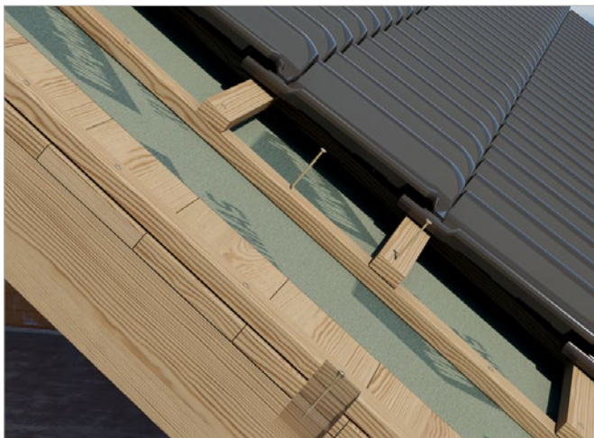
Fixing of battens and counter battens
